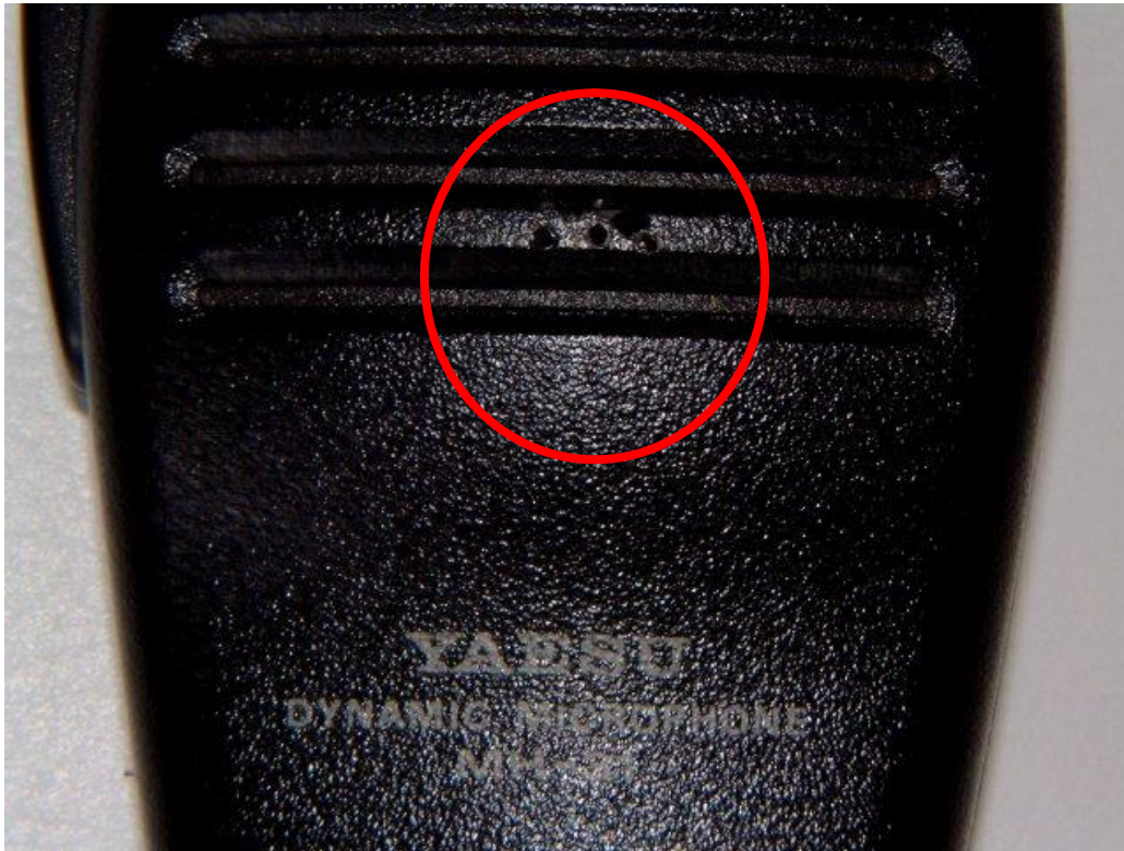
Turning some small holes in the middle of the new capsule position to give a better audio input.
